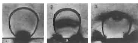
Figure 2.7 Radial jetting during water drop impact (photographs: Camus, 1971).
