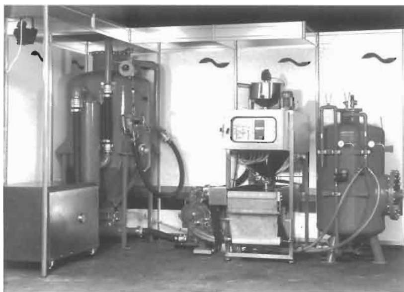
Figure 3.30 Modular water treatment system for hydroblasting applications (WOMA Apparatebau GmbH, Duisburg).
