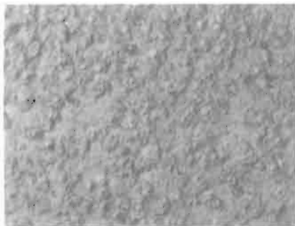
Figure 6.2 Examples for initial conditions of a plain steel and a previously coated surface (STG 2222).
