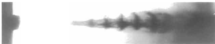
Figure 7.9 Appearance of a self-resonating water jet, v_j = 83.8 m/s, f_p = 4.6 kHz (photograph: Dynaflow ® Inc., Jessup).
