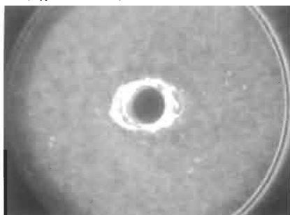
Figure 3.22 Characteristic wear types in hydroblasting sapphire nozzles.
